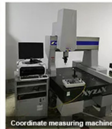
Coordinate measuring machine
